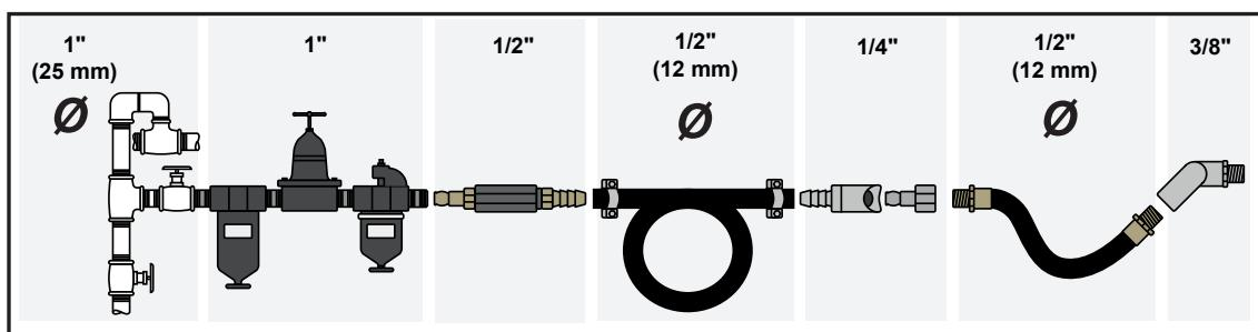
**Figure 01****Max. air pressure = 6.3 bar**
